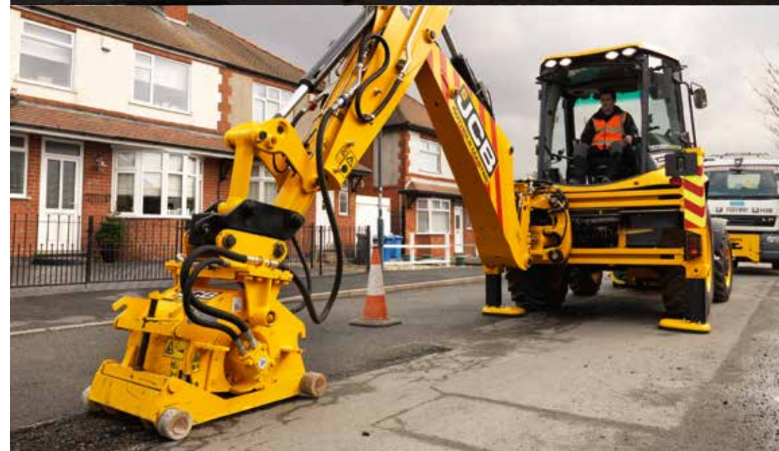
2. START PLANNING | Precise planning up to a depth of 115mm.
